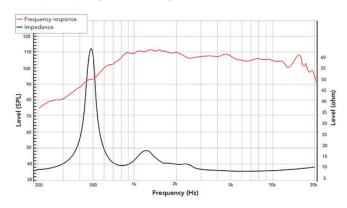
Frequency response measured on IAC baffle
