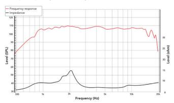
Frequency response measured on IAC baffle
