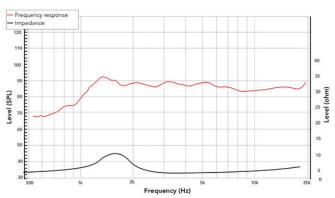
Frequency response measured on IAC baffle
