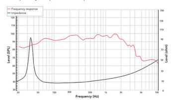
Frequency response measured on IAC baffle
