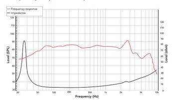
Frequency response measured on IAC baffle
