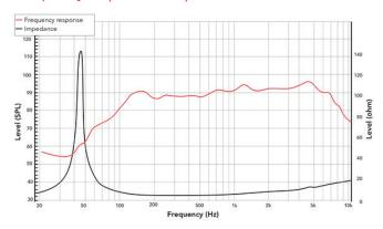
Frequency response measured on IAC baffle
