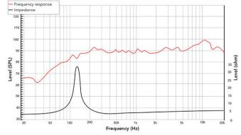
Frequency response measured on IAC baffle
