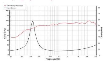
Frequency response measured on IAC baffle
