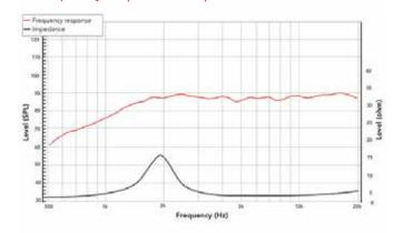
Frequency response measured on IAC baffle
