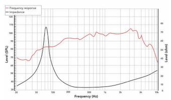
Frequency response measured on IAC baffle
