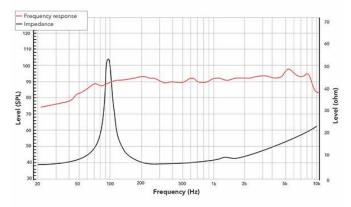
Frequency response measured on IAC baffle
