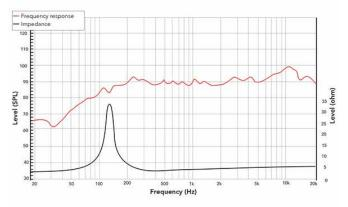
Frequency response measured on IAC baffle
