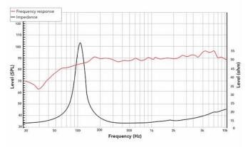
Frequency response measured on IAC baffle
