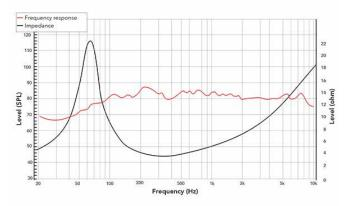
Frequency response measured on IAC baffle
