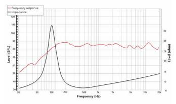
Frequency response measured on IAC baffle
