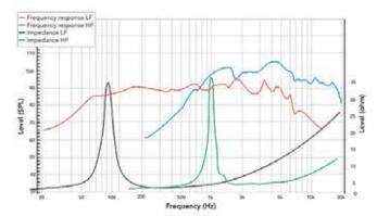
Frequency response measured on IAC baffle
