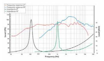
Frequency response measured on IAC baffle
