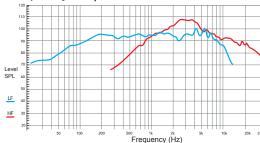
Frequency response measurement with transducer mounted on IEC half space baffle.
