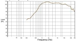
Frequency response measurement with transducer mounted on constant directivity horn
