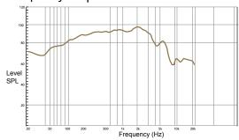
Frequency response measurement with transducer mounted in a 40 liter vented enclosure tuned to 65Hz
