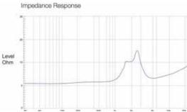
Impedance measured in free air without a horn
